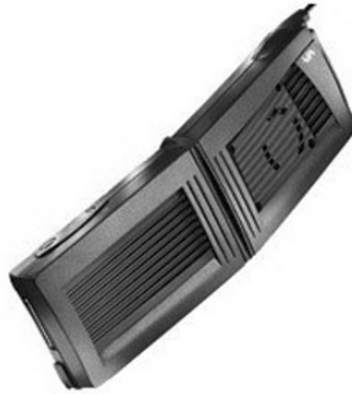
Fig. 5-14. Segmented Computer Form Factor (For more information on Infologix Via wearable computer go to www.infologixsys.com )
