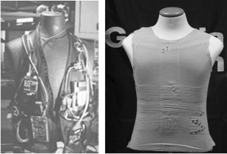
Fig. 4-3. Hosting a Distributed Wearable Systems in a Single Garment. Left: MIThril wearable system (MIT Media Lab/Alex Pentland), right: GATech Smartshirt (Courtesy: Textile Information Systems Research Laboratory, Georgia Institute of Technology, Atlanta, Georgia, USA)
