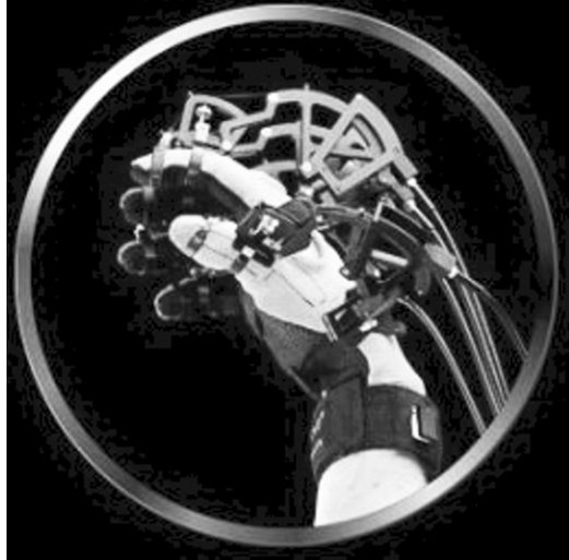
Fig. 9-2. The Cybergrasp Force Feedback Glove (Reproduced by permission of Immersion Corporation, Copyright ©2006 Immersion Corporation. All rights reserved)
