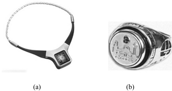
Fig. 3-4. Jewelry with Embedded Electronics: (a) Nokia Medallion (courtesy Nokia Corp), (b) iButton® (photo courtesy of Dallas Semiconductor)
